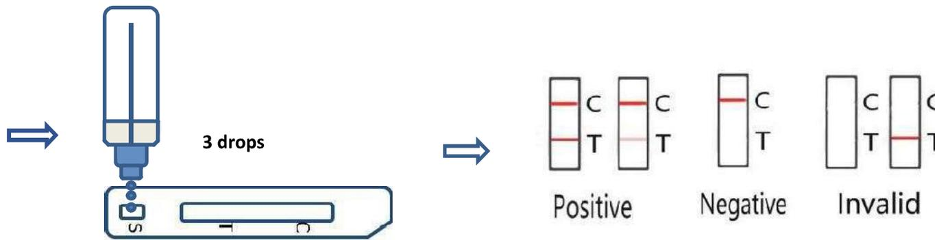
10. Add 3 drops of the sample into the sample hole vertically
